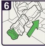
· Hold the lever and push in the cartridge.
