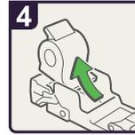
· Remove the empty refill in the direction of the arrow.
