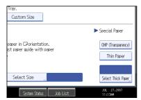
5. Select the paper type (one of [Thick Paper 1], [Thick Paper 2], and [Thick Paper 3]), and then press [OK].
