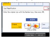
You can enter sizes between 1 to 999 mm (0.1 to 99.9 inches) in increments of 1 mm (0.1 inch).
