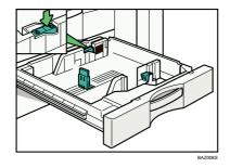
4. While pressing down the release lever, slide the side fences until they are aligned with the paper size you want to load.
