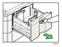
Load paper into the paper tray by pushing the paper to the left side of the paper tray. Place paper with printing side up.
