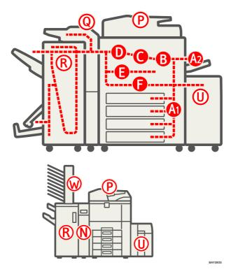
1. Press the key of the section from where you want to remove the jammed paper.
