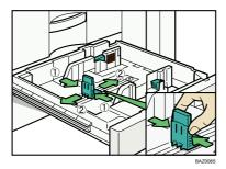
6. While pinching the sides of the end fence, slide it into position according to the paper size you want to load.
