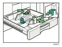
5. While pinching the sides of the end fence, slide it a little to release the lock.
