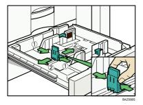
6. Slide the end fence into position according to the paper size you want to load.
