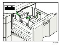
7. Tightly fit the back fence to the loaded paper and then re-lock the back fence again.
