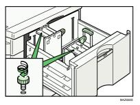
5. Release the lock on the back fence.
