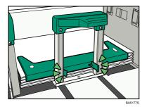
• When loading paper size which is smaller than that of envelope, set the Postcard Side Fence in the Wide LCT.
