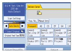
2. Using the number keys, enter the three-digit registration number, and then press the [#] key.
