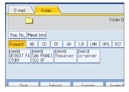
2. Enter the five-digit registration number that has been assigned to a destination folder using the number keys.
