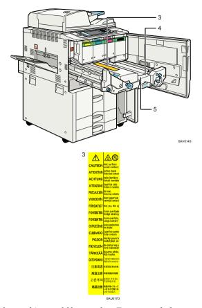
The inside of the machine could be very hot. Do not touch the parts which a label is put on. Otherwise, an injury might occur.
