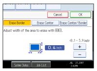
Pressing [+] or [-] changes the width in increments of 1 mm (0.1 inch). Pressing and holding down the relevant key changes the width in increments of 10 mm (1 inch).
