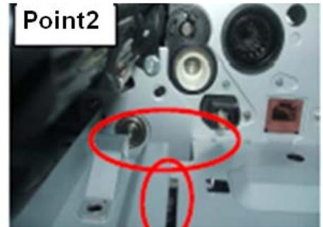
10. Remove the ring clip on the Y toner supply unit with a pair of tweezers.
