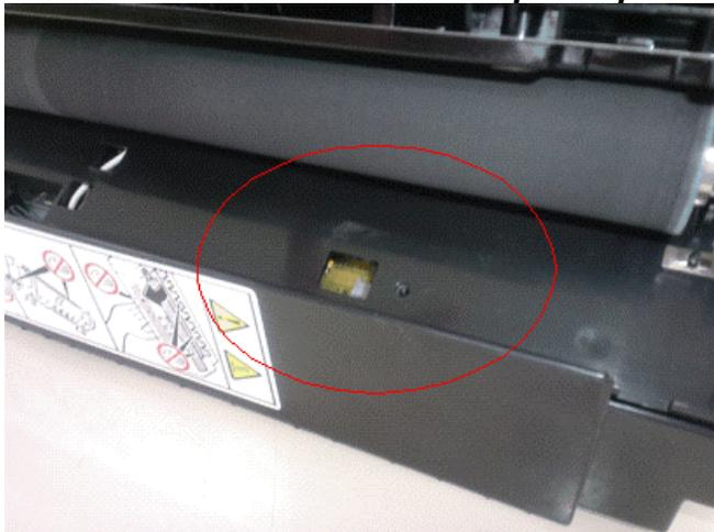
2. **Make sure the screw for the ground plate, circled in red below, is properly tightened.**
