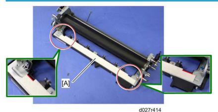
Attach the fusing cleaning felt [A], aligning both edges of the fusing cleaning felt with the red lines on the bottom cover.
