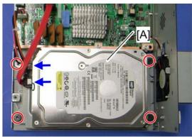
2. Remove the HDD [A] with the bracket ( $\hat{\mathscr{E}} \times 4$ ,  $\mathbb{Z} \times 2$ ).
