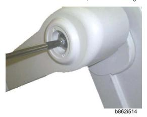
5. Secure the handle unit with a screw ( $\mathscr{F}$  x 1: M3x8).
