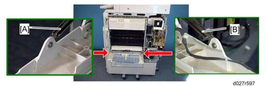
9. Release the front [A] and rear [B] arms ( $\langle\!\!\langle\bar{\rangle}\!\!\rangle$  x 1 each).
