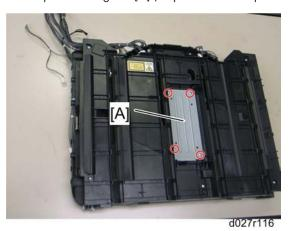
2. Polygon mirror motor cover [A] of the laser optics housing unit (  $\hat{\mathscr{F}} \times 4)$
