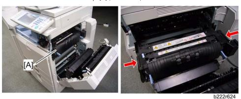
5. Pull out the fusing unit [A].
