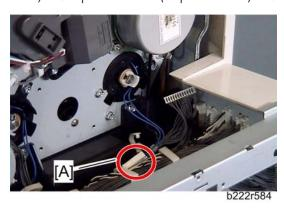
5. Disconnect the connector [A] (□ x 1).
