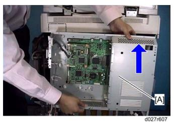
10. Lift up the controller box [A], and then remove it.
