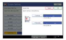
Press [Horizontal], enter the horizontal size of the paper using the number keys, and then press the [<sup>#</sup>] key. 9. Press [OK].
