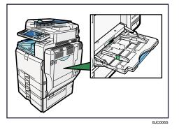
2. Gently insert paper face up into the bypass tray until the beeper sounds, and then adjust the paper guides to the paper size.
