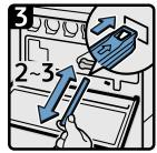
3. There are four holes for cleaning 4. Slide the cleaning brush in and out slowly 2 to 3 times to clean all four areas.
