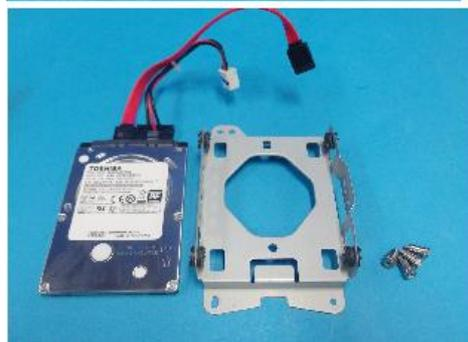
5. Disconnect the cables from the standard HDD. ( x 2)
