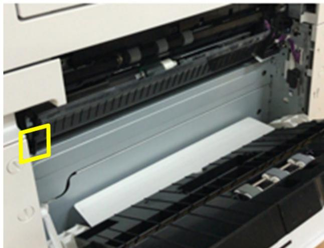
2. Attach the guide plate by sliding it toward the right hole.
