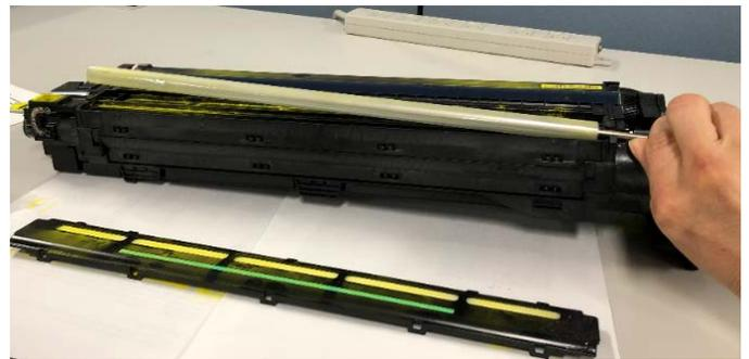
3. Insert the Mylar into the **slit** of the upper cover.
