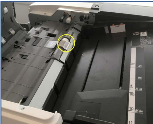
3. Remove the paper feed guide plate.
