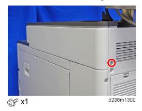
3. Remove the scanner right cover [A].
