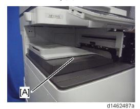
6. Remove the paper exit feeler [A] to apply the Mylar sheet properly.
