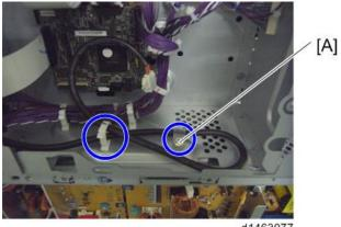
9. Connect the key counter's cable to the 4-pin connector [A] on the machine.
