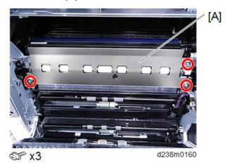
4. Remove two screws, then release the tab by inserting a flathead driver behind the registration sensor [A].
