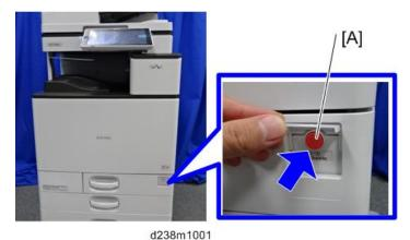
2. The shutdown message appears. After the shutdown process, the main power is turned off automatically.
