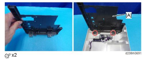
5. Remove the scanner front cover [A].
