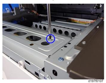
15. While pressing the bottom plate [A] into the area shown by the blue circle [B], insert it into the slot shown by the blue circles [C] [D].
