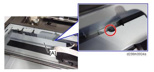
25. Connect the heater harness that was pulled out of the frame hole to the connector which was mounted in step 15.
