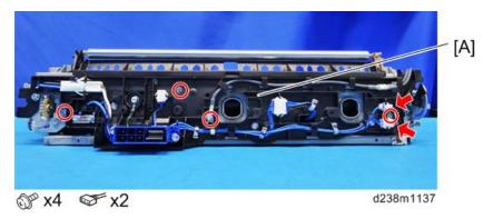
4. Fusing sleeve thermostat unit [A]
