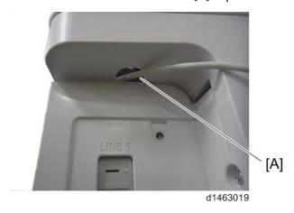
14. Connect the USB connector to the USB interface of the controller.
