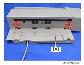
5. Place the slide rail [A] under the internal finisher [B].
