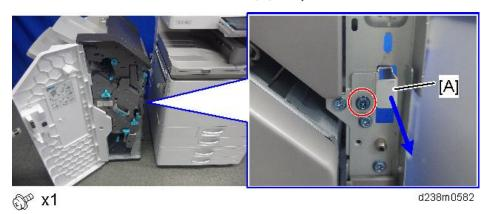
15. Connect the finisher to the main unit, and then push in the connection lever [A] to fasten it to the main unit. ( x1)
