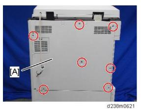
10. Remove the small disposable cover [A] on the rear cover (on the right side).
