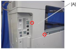
9. Remove the inverter tray [A], and tray support rod cover [B] (50°×1).
