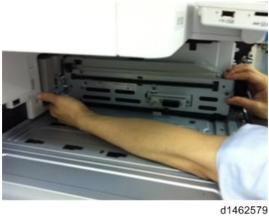
8. When installing the punch unit in a finisher that is already installed, remove the relay guide plate [A] (\$\mathbb{O}^\* \times 2\$).
