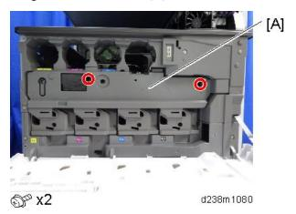
3. Release the ITB lock lever [A].
