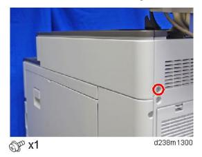
3. Remove the scanner right cover [A]
