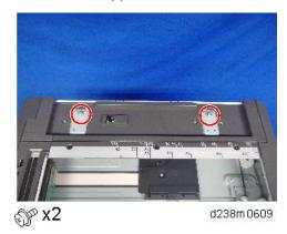
5. Align the hinges of the SPDF with the stepped screws, and attach them by sliding them in.
