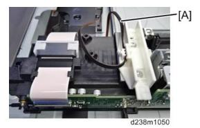
8. Lower the lock lever [A] and disconnect the FFC [B].
