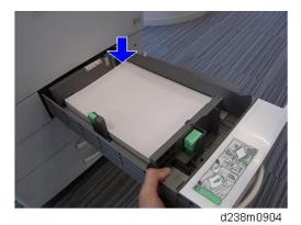
4. Reattach the tray. Lift the tray slightly when you attach it.
