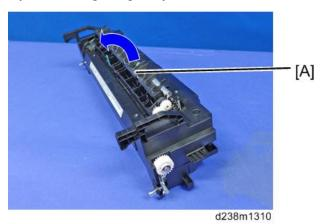
2. Wipe clean with a dry cloth. Then wipe clean with a cloth dampened with alcohol.
