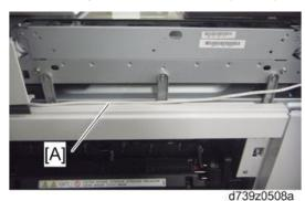
12. Route the keyboard cable along the rear side of the scanner unit (\$\varphi x 1).
