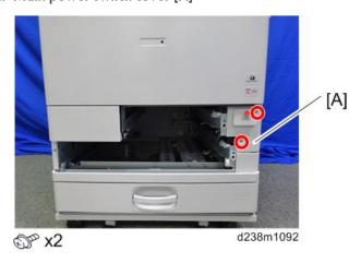
3. Insert a screwdriver through the hole in the frame, and detach the temperature and humidity sensor together with its bracket [A].
