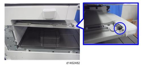
17. Insert the tray support bar firmly in the 1-bin tray, and attach the harness cover [A].
