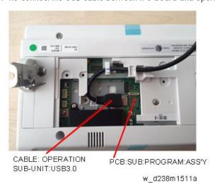
When connecting the cable, hold the molded part of the cable as shown below so as not to apply excessive force on the connector part. Applying excessive force toward the upper direction on the connector may cause connection failure.
