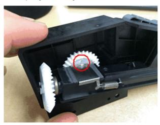
1. Before installing, check that the lever on the image transfer lock unit is in the unlocked position.
