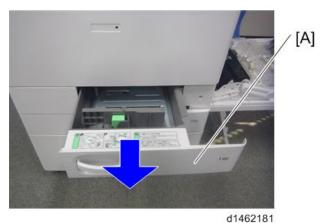
5. Press the left tab to release the lock, and remove the paper feed guide plate [A].
