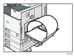
• When using paper that has a horizontal width of 900 mm (35.5 inches), curl the paper so that its leading edge touches the side of the machine.
