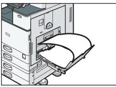
• When using paper that has a horizontal width of 457.2-900 mm (18.00-35.5 inches), set the paper so that its leading edge protrudes from the banner paper guide tray.
