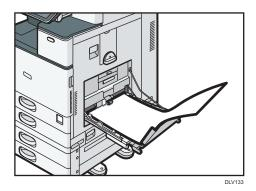
When using paper that has a horizontal width of 148–457.2 mm (5.83–18.00 inches), set the paper as loading paper into the bypass tray.
