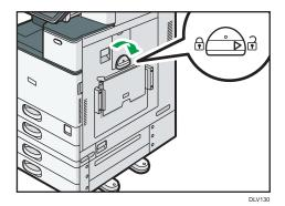
1. Turn the knob clockwise until its triangle mark stops at the unlock mark.
