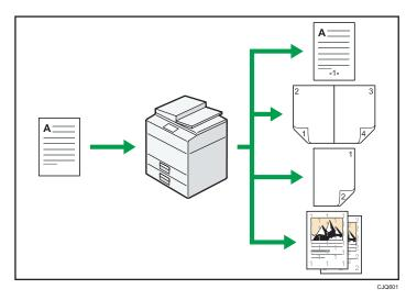
• You can make copies in full color. You can switch the color copy mode depending on the type of originals used and the desired finish.
