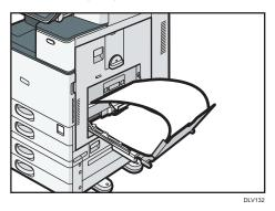
• When using paper that has a horizontal width of 457.2–900 mm (18.00–35.5 inches), set the paper so that its leading edge protrudes from the banner paper guide tray.
