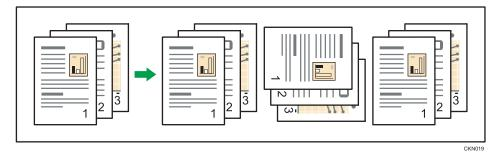
To use the Rotate Sort function, two paper trays loaded with paper of the same size and type, but in different orientation (DD), are required. For details, see "Tray Paper Settings", Connecting the Machine/ System Settings.
