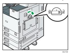
2. Hold the handle in one hand while supporting the back of the bypass tray with the other hand, and then open the bypass tray slowly.
