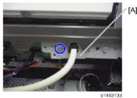
10. Remove the ADF (screws x 2)
