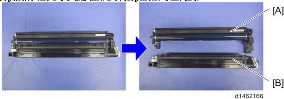
7. Rotate the PCU unit and remove the charge roller unit (⚙️×2).
