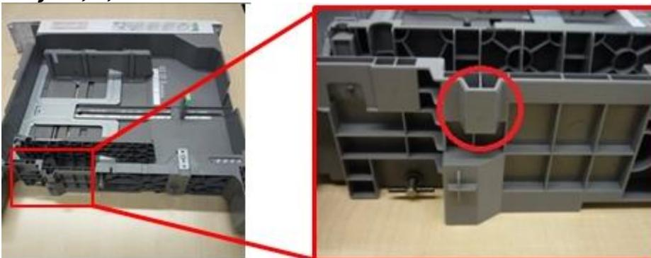
4. Attach the spacer as shown in the diagram.
