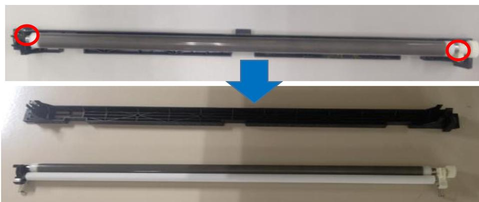
9. Re-attach the charge roller and charge roller cleaning unit together with the new frame and new plate.
