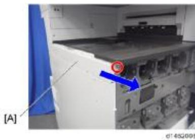
3. Remove the left rear cover [A] (screws x 2)
