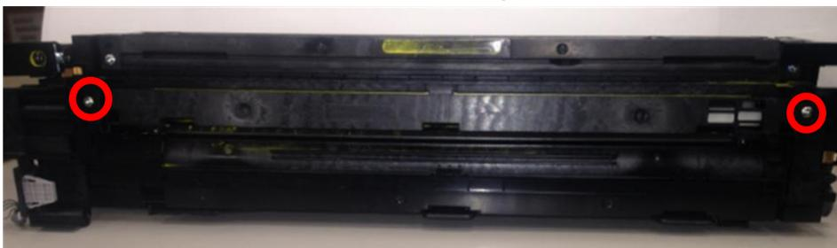
8. Remove the charge roller and charge roller cleaning unit (hook x2).
