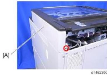
12. Remove the scanner front cover [A] (screws x 2)
