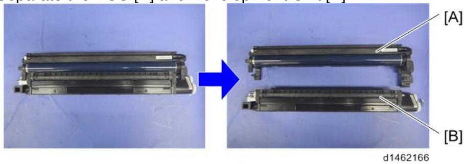
7. Rotate the PCU unit and remove the charge roller unit (⚙️ x2).
