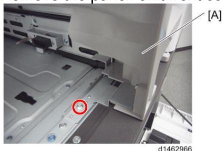
9. Remove the punch unit [A] (x1).
