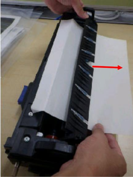
12. Repeat Steps 6 and 7 until the gap between the exit guide plate and fusing upper cover is 2.5mm or more.
