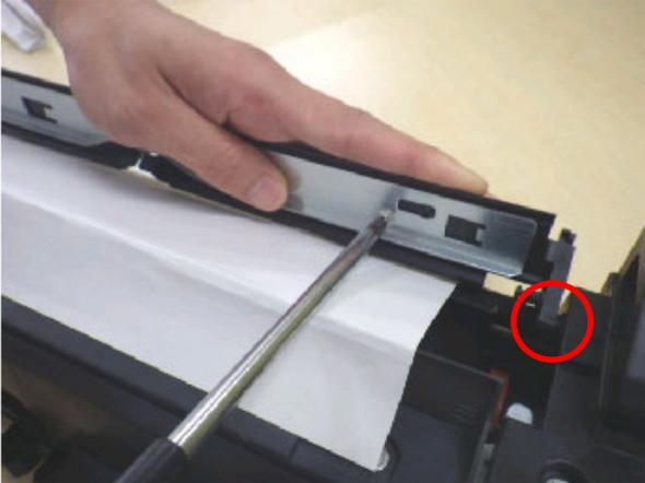
8. Slide the metal plate in the direction shown by the red arrow and remove the plate.
