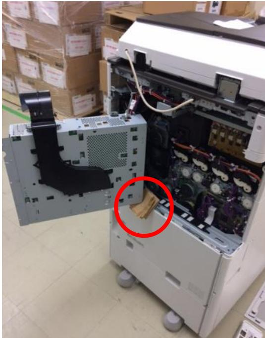
8. Remove the imaging IOB [A] ( ×5, ×14).
