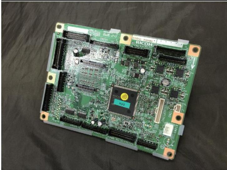
12. Reinstall the imaging IOB.
