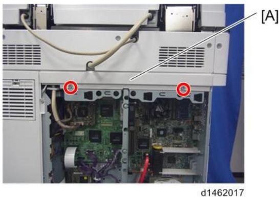
17. Reinstall the scanner rear cover [A] ( ×3).
