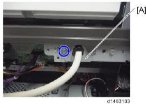
10. Remove the ADF (screws x 2)
