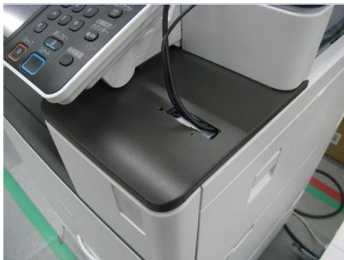
19. For D197-D202 ONLY: Attach the Shift Bracket.
