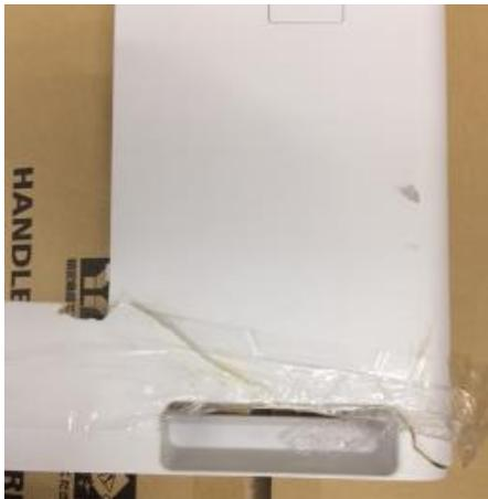
Figure.4 Broken right rear cover
