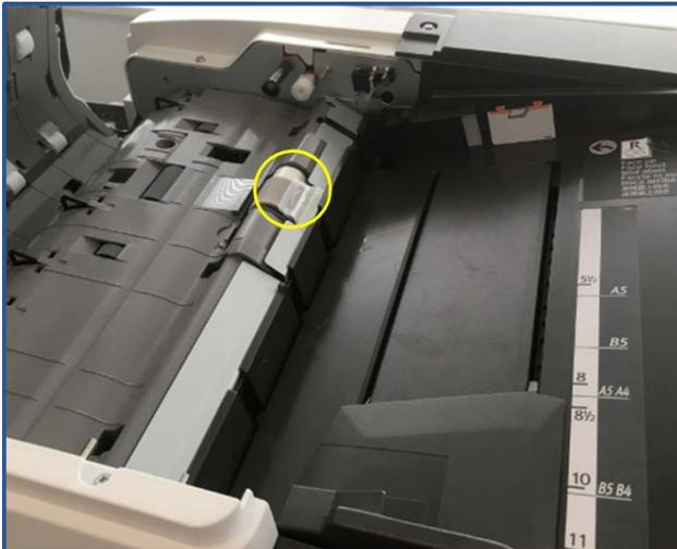
3. Remove the paper feed guide plate.
