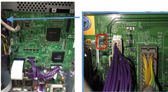
**Figure 7: Fuse on the IPU**
