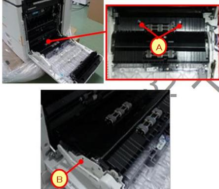
6. Remove the cover by releasing the hook shown by the red arrow and remove the screws [A].
