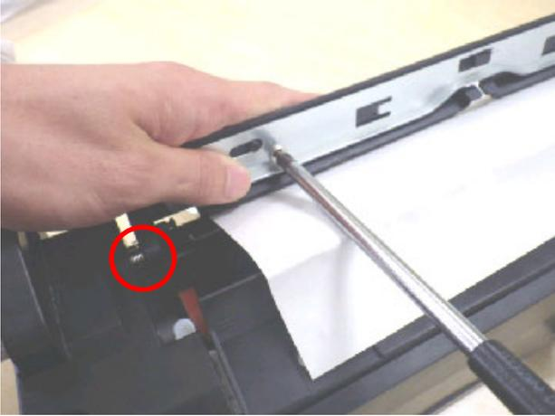
4. Collect the small metal shavings (from when the screw was removed) onto the paper, as shown below. Repeat this 5-10 times.
