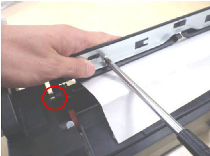
4. Return the fusing unit to the machine.
