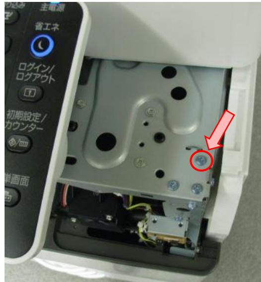
5. Attach the clamps (x3) to the right hand side of the scanner unit.
