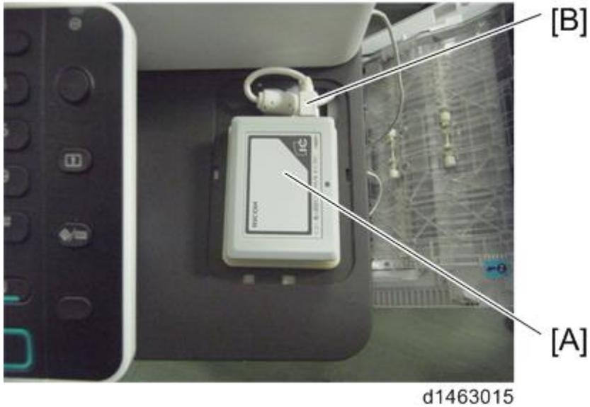
**IMPORTANT:** Twist the USB cable before attaching it as shown in the photo.
