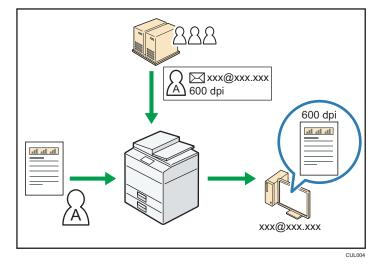
• You must set up and configure a Windows server to use the distributed scan management system. This system is supported under Windows Server 2008 R2.
