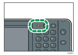
• When using the Smart Operation Panel Press [Reset] on the top right of the screen.
