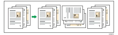
To use the Rotate Sort function, two paper trays loaded with paper of the same size and type, but in different orientation ( $\square\square$ ), are required. For details, see "Tray Paper Settings", Connecting the Machine/ System Settings.
