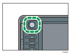
• When using the Smart Operation Panel Press the [Home] key on the top left of the control panel. Flick the screen to the left, and then
