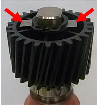
2. Permanent solution: The inside diameter of the pressure roller gear was changed to decrease the gaps.
