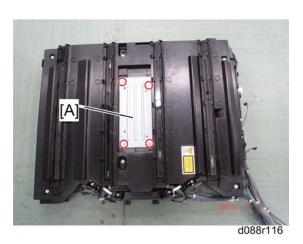
2. Polygon mirror motor cover [A] of the laser optics housing unit (  $\rlap{/}{P} \times 4)$
