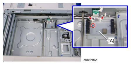
3. Original length sensor bracket [A] ( F x 1, III x 2, III x 2)
