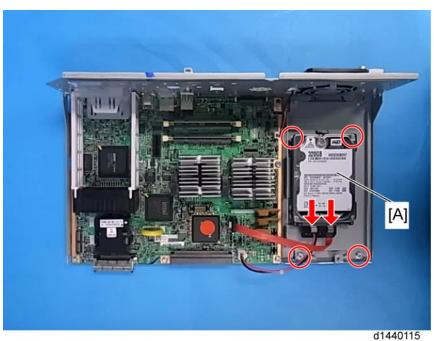
2. Remove the HDD [A] with the bracket (  $\mathscr{F}$  x 4,  $\mathbb{I}^{2}$  x 2).
