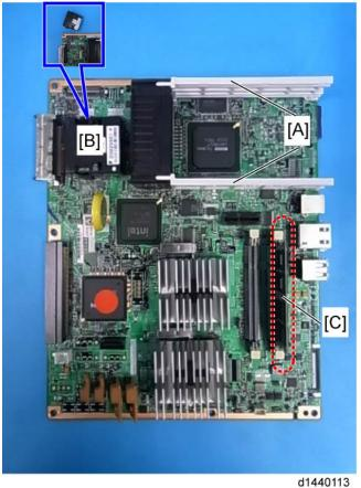
3. Interface rails [A], NV-RAM [B], RAM-DIMM [C]
