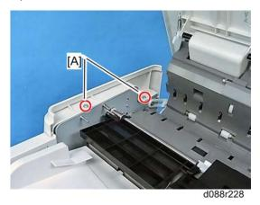
2. Remove two screws  $\left[A\right]$  on the front cover.
