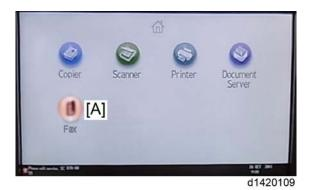
If the fax icon is not displayed (as shown below), the FCU should be replaced. Refer to the Fax service manual for the FCU replacement procedure.
