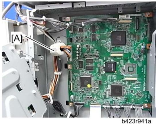
75 Install the core [A] (TFC16816) in the harness of CN110 (on the BICU).
