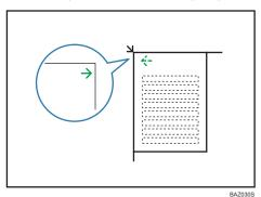
Make sure to set the test pattern on the exposure glass, and then two or three white sheets, same size
