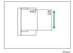
• If you do not select [Mixed Original Sizes] and place originals of different sizes in the ADF, paper jams might occur or parts of the originals might not be scanned.
