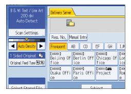
The selected destination is highlighted and also is displayed in the destination field at the top of the screen.
