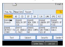
The key of the selected destination is highlighted, and the destination appears in the destination field at the top of the screen.
