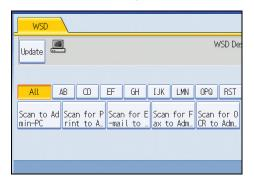
The key of the selected destination client computer is highlighted, and the destination appears in the destination field at the top of the screen.
