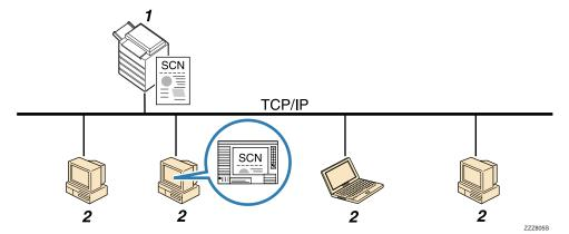
Scans an original after receiving a scan instruction from a client computer, and then sends the scan file over the network to the client computer.
