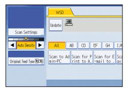
Note that only [Erase Border] can be specified directly from this machine. Use the client computer to configure the other scan settings. For details, see "Changing a Scan Profile".
