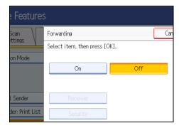
If there is an End Receiver already programmed, a receiver name is shown. If you want to change the receiver, press [Receiver] and proceed to step 5.
