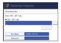
To change the SEP Code, press [Clear], and then try again. To change the box name, press [Box Name], and then repeat the procedure from step 7.
