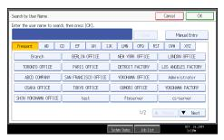
To search by directly entering a user name, press [Manual Entry], and then enter the user name. Forward matching is used when searching for a user name.
