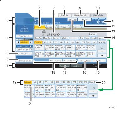
1. Displays the date, time, and machine status. Displays the name, facsimile number of the destination, and the size of the original when transmitting.
