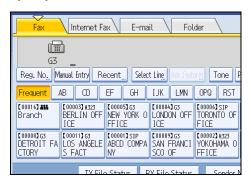
Press the transmission type tab to switch the transmission type between fax/IP-Fax, Internet Fax, email, and folder.
