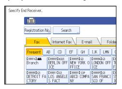
Press the transmission type tab to switch the destination between fax number, Internet Fax destination, e-mail address, and folder destination.
