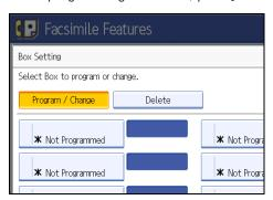
To change a box already programmed, press it, and then proceed to step 8. If a password is programmed, enter the password, press [OK], and then proceed to step 8.
