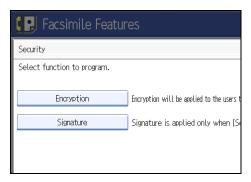
To specify encryption for documents for transfer to receiving station, press [Encryption]. To use the encryption function, the address must be stored in the Address Book and have the encryption option enabled. For details about Encryption, consult your administrator.
