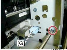
21. Remove the paper dust case [G] and two screws (at the front and rear frame each).
