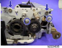
9. Upper frame [G] ( $\mathscr{F}$  x 5, stepped screw x 3, stud screw x 1)
