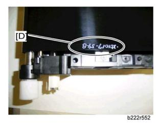
• This belt must be installed the correct way around. When you reinstall the image transfer belt unit, install it with the painted number [D] on the belt at the rear side of the unit.
