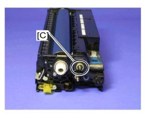
5. Remove the bushing [C] of the development roller at the rear of the PCU ( $\mathbb{C} \times 1$ ).
