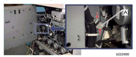
4. Disconnect the connector [A] ( x 1)
