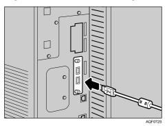
Secure the USB cable using the hook.
