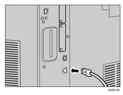
**4** Connect the other end of the Ethernet cable to a network connection device such as a hub.
