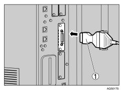
Use the conversion connector (1) supplied with the IEEE 1284 interface board.
