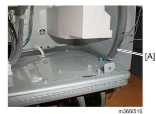
12. Make sure that the harness (harness 1) [A] is placed securely as shown above.
