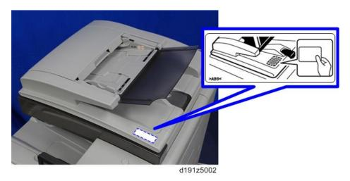
7. Attach the location decal to the front-right on the ARDF.
