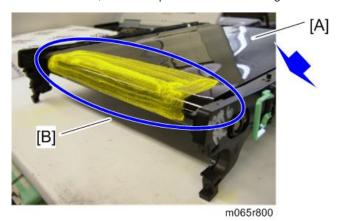
1. Lubricate a part of the surface of the image transfer belt [A] with yellow toner, and then turn the image transfer belt to the position [B] as shown above.
