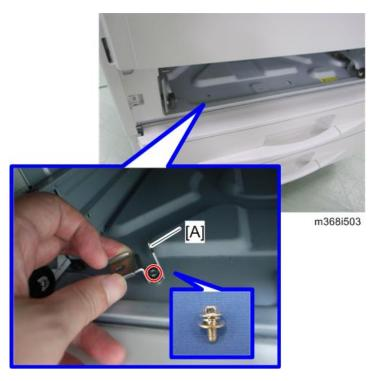
5. Attach a screw (spring washer screw), using a securing bracket [A] to tighten the screw.
