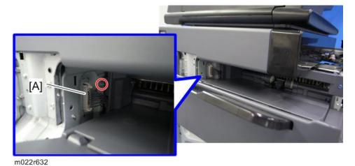
6. Disconnect the harness [A] and remove the screw.
