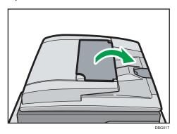
2. Place the aligned original face up into the ADF, and then adjust the document guides to the original size.
