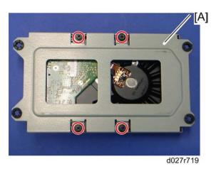
3. Remove the HDD from the bracket [A] ( $\mathscr{F} \times 4$ ).
