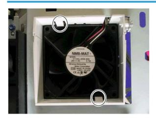
Make sure that the fusing/paper exit fan is installed with its decal facing to the right side.
