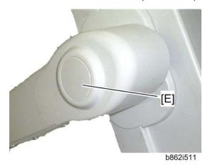
6. Clean the handle unit with alcohol. Then attach the stud decal [E] at the location that was cleaned.
