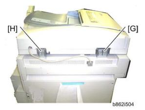
9. Attach the hinge stoppers (left [G] and right [H]) to the left and right hinges (Tapping screw x 2: M4x8 each).
