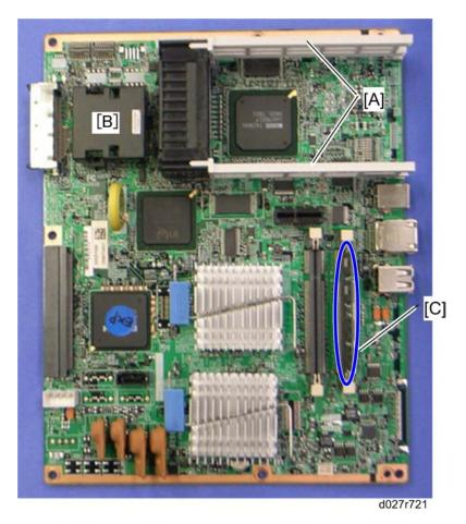
3. Interface rails [A], NV-RAM [B], RAM-DIMM [C]
