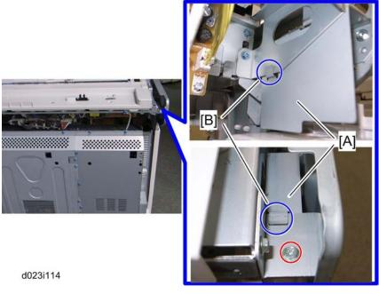
12. Attach the bracket [A] with its two hooks [B] as shown above ( $\hat{\mathcal{E}}$  x 1: M3x6).
