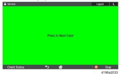
The check is completed when all colors have been displayed. The screen returns to the top menu of [Self Check].
