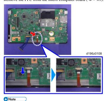
• Pull out the black part to unlock the connector, and then remove the FFC.
