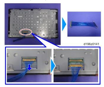
Remove the tapes for fixing the microphone harness (tape  $\times$ 3).
