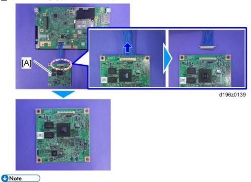
• After replacing the CPU board, make sure that the latest version of the firmware is installed on the Smart Operation Panel. Update it if necessary. (Updating the Smart Operation Panel)
