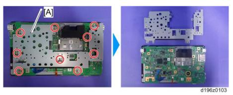
4. Remove the fixing screws ( x4) on the CPU board [A], and remove the CPU board from the micro
