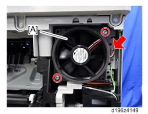
3. Remove the cover from the fusing fan [A].
