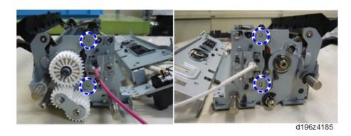
• The fusing sleeve belt assembly for replacement has a jig [A], which must be removed. Set the fusing sleeve belt assembly first, tighten the screws, then remove the jig.
