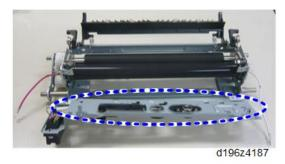
• When reattaching the fusing sleeve belt assembly, do not let the fusing sleeve belt assembly hit the projection of the sensor or the screws on the stay.
