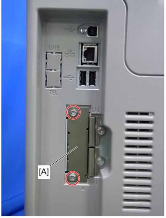
1. Remove the slot cover [A] from the board slot (  $\mathcal{F} \times 2$  ).
