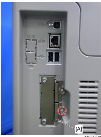
1. Remove the slot cover [A] for the SD card (  $\rat{p} \times 1$  ).
