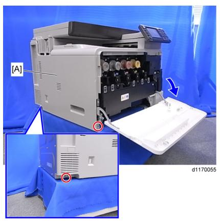
2. Open the front cover and remove the left cover [A] (  $\slash\hspace{-0.6em}P \times 2).$
