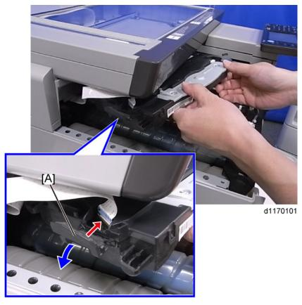
4. Open the connector cover [A], release the lock and disconnect the flat cable.
