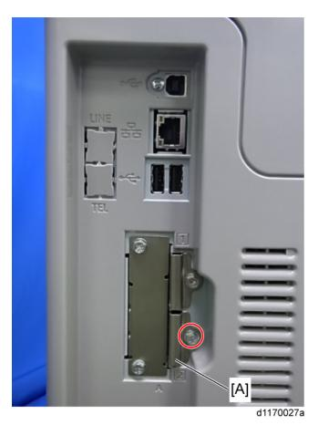
2. Remove the slot cover [A] (  $\mbox{\it P} \times 1$  ).
