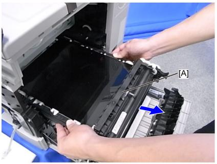
7. Remove the ITB unit [A] while holding the right and left guides of the unit.
