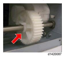
5. Snap attached beside the gear (snap x 1)
