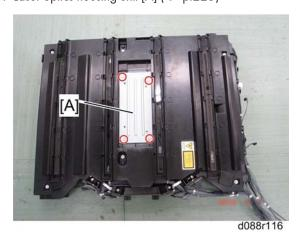
2. Polygon mirror motor cover [A] of the laser optics housing unit (  $\mbox{\ensuremath{\not{p}}}\xspace x 4)$
