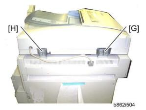
9. Attach the hinge stoppers (left [G] and right [H]) to the left and right hinges (Tapping screw x 2: M4x8 each).
