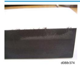
The fusing entrance guide plate requires cleaning maintenance every fusing unit maintenance interval. Clean the fusing entrance guide plate at the place shown above with a dry cloth, and then clean the fusing entrance guide plate again with a cloth moistened with alcohol.
