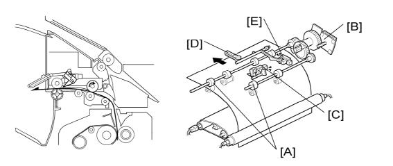
The paper exit rollers [A] feed paper to the standard tray. These rollers are driven by the fusing/paper exit motor [B].
