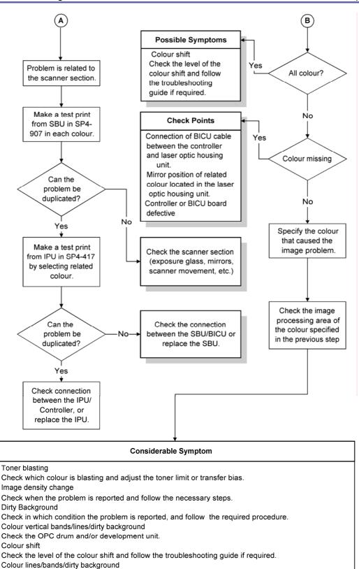
When the PCU/development unit is close to its life end, the developer or the cleaning blade of the PCU wears out, causing vertical colour lines, bands, or dirty background. Check the related colour unit and replace it if necessary.
