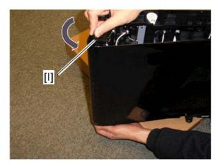
12. Pull the tension roller [I] as shown.
