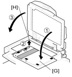
9. Peel off the platen sheet [G] and place it on the exposure glass.
