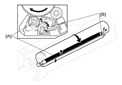
This machine uses a non-contact charge roller [A] to reduce ozone. The non-contact charge roller gives the drum surface a negative charge. The high voltage supply board – C.B, which is located at the rear of the machine, applies a dc and ac voltage (at a constant current) to the roller. The ac voltage helps to ensure that the charge given to the drum is as uniform as possible.
