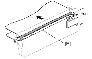
Finally, the discharge plate [E], which is given an AC charge, discharges the paper.
