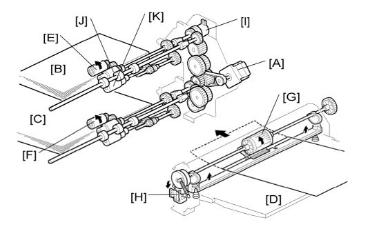
The paper feed motor [A] drives the pick-up and feed mechanisms in tray 1 [B], tray 2 [C]. It uses clutches and complex trains of gears to do this.
