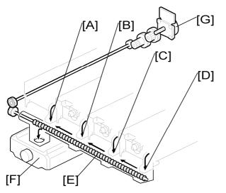
The used toner from the collection augers in the four PCUs drops into the toner collection duct from the four openings [A][B][C][D] at the front of the PCUs. The toner collection auger [E] in the duct transports this used toner towards the toner collection bottle [F]. The coil [E] is driven by the toner transport motor [G]. The openings and PCUs correspond as follows: Yellow  $\Rightarrow$  [A], Cyan  $\Rightarrow$  [B], Magenta  $\Rightarrow$  [C], Black  $\Rightarrow$  [D].
