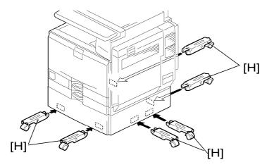
9. Attach the two caster stands [H] to front, left, and rear sides of the machine.
