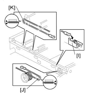
6. Hook the right end onto the front scanner wire bracket [I]. The end should go via
