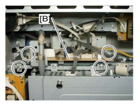
3. SIO board with bracket [B] ( x 4, All Iss)
