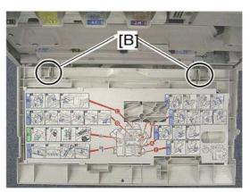
2. Remove the two pins [B], and then remove the front cover.
