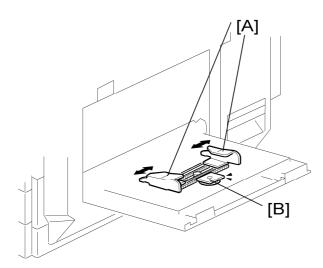
There are two paper side plates [A] on the by-pass tray. These connect with the paper size sensor [B] through a rack-and-pinion mechanism.
