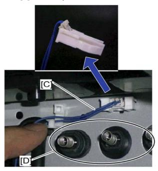
4. Connect the harness [C] to the connector of the machine.
