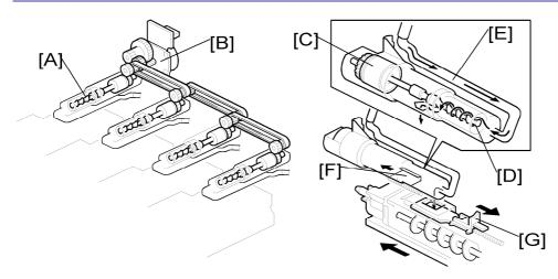
Each toner attraction pump [A] is driven by the toner transport motor [B]. Each toner attraction pump has the same mechanism. The pump (toner attraction pump) has the following components:
