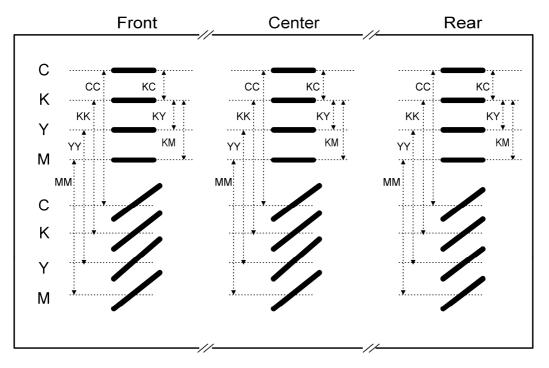
During automatic line position adjustment, the line patterns above are created eight times on the transfer belt. The spaces between the lines (CC, KK, YY, MM, KC, KY, KM) are measured by the front, center, and rear ID sensors. The controller takes the average of the spaces. Then it adjusts the following positions and magnification:
