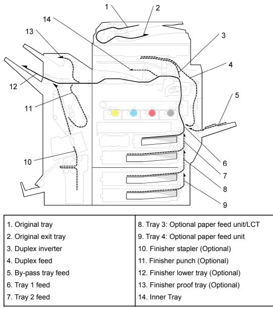
The 1000-sheet finisher and 1000-sheet booklet finisher require the bridge unit (B227) and one from the two-tray paper feed unit (B800) or the LCT (B801).
