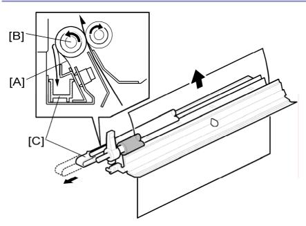
The two mylars [A] scrape the paper dust from the registration idle roller [B]. The paper dust falls down into the paper dust container [C].
