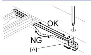
Run the cable so there is no slack. Slide the clamp [A] to adjust the cable slack.
