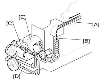
The toner collection auger [A] moves the used toner from the image transfer belt and the used toner drops into the toner collection duct [B]. The toner collection coil [C] moves the used toner to the opening [D] at the rear of the toner collection bottle. The toner transport motor [E] drives the toner collection coil.
