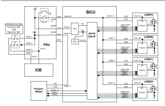
A relay on the PSU ensures technician and user safety. It also prevents the laser beam from turning on during servicing. This relay turns off when the front cover, upper left cover, or right door is opened. At this time it cuts the power (+5V) supplied to the LD board for each color through the BICU.
