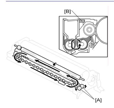
Two mixing augers [A] circulate the developer forward and backward to agitate the developer. This happens at the following times:
