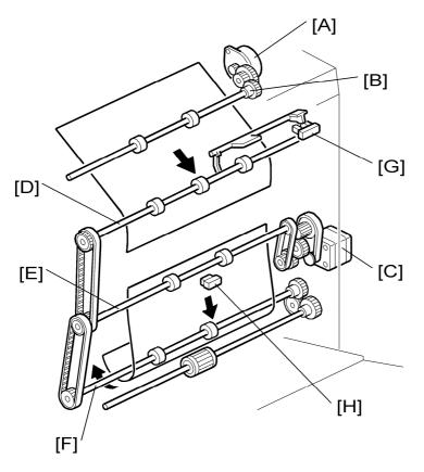
The duplex inverter motor [A] drives the following:
