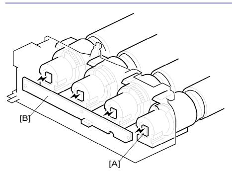
Each toner cartridge of this machine has a RFID chip [A]. This stores the total "on" time of the toner supply clutch. This is used to calculate the amount of toner remaining in the toner cartridge. The chip is also used to detect whether the cartridge is installed (if the cartridge is not installed, the machine does not detect a signal from the memory chip). The RFID transmits its data to the RFID antenna board [B] without any contact.
