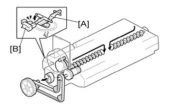
The toner collection bottle has a projection at its rear side. When the toner collection bottle is set, this projection pushes the waste toner bottle set switch at the rear of the machine. As a result, the machine detects that the toner collection bottle is installed.
