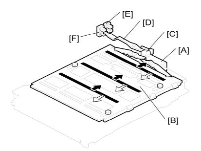
The laser optics housing unit has a shutter. As a result, toner and other dust do not fall on the glass of the laser optics housing. The shutter motor [A] moves the shutter [B] in the direction of the arrow with the cam [C] (to open: black arrow direction, to close: white arrow direction). First, the actuator [D] stays at the shutter closed sensor [E]. The shutter motor opens the shutter and the actuator moves to the shutter open sensor position [F] after the polygon motor has turned on.
