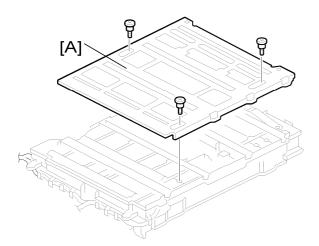
1. Shutter [A] of the laser optics housing unit ( x 3)
