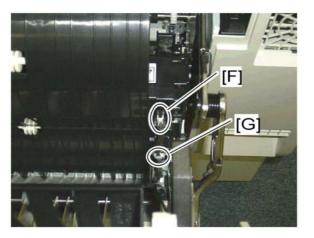
7. Disconnect the connector [F] and release the clamp [G].
