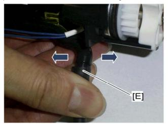
8. Slowly remove the toner supply tube [E] from the toner pump unit by pulling the tube right and left.
