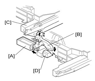
This mechanism is only activated when the machine detects a paper jam. The lock at the rear prevents the tray from coming out from the machine when the paper is jammed. If the tray is removed while the paper is jammed, the paper may be split in two pieces. This makes it difficult to remove the jammed paper.
