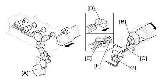
The toner transport motor [A] rotates the toner bottle-Bk via gears and a clutch. It also rotates the toner bottle-Y, -C, -M via gears, clutches and timing belts.
