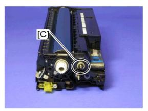
5. Remove the bushing [C] of the development roller at the rear of the PCU ( $\ensuremath{\mathbb{C}}$  x 1).
