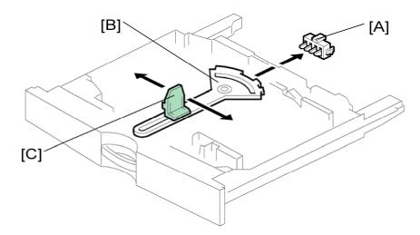
There is no size switch for tray 1. The paper size is fixed at either A4 or LT (LEF for both sizes). You can change the size setting with SP5-181-1.
