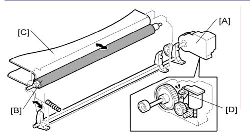
The paper transfer contact motor [A] keeps the paper transfer roller [B] in contact with the image transfer belt [C]. This motor has the paper transfer HP sensor [D] inside. The paper transfer HP sensor detects if the paper transfer roller is in contact with the image transfer belt. Only when the machine executes the line position adjustment or process control, the paper transfer unit keeps away from the image transfer belt.
