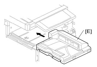
7. Install the bridge unit [E] in the machine.
