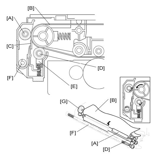
The ITB-cleaning unit removes toner (during printing) and the ID sensor patterns (during process control or automatic line position adjustment) on the belt. Belt cleaning is completed while the image transfer belt makes one rotation. The ITB drive motor drives the ITB-cleaning unit.
