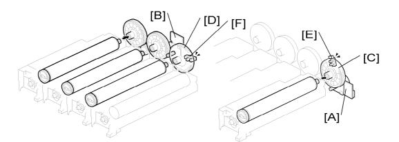
The drum/development drive motor-K [A] drives the drum unit for black. The drum drive motor-CMY [B] drives the drum units for magenta, cyan, and yellow. Using one motor to drive these three drums reduces CMY color misalignment. Both motors are brush-less DC motors. This helps to reduce the drive noise.
