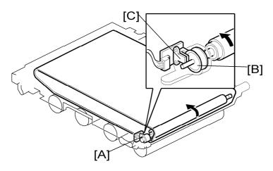
This machine uses the rotation encoder to control the transfer belt speed.
