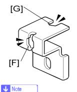
One of the securing brackets is used as a securing tool (the cutout [F] is used in step 6). But the cutout [G] is for attaching the tray heater. Therefore, attach the securing brackets [E] after installing the tray heater if you will install the tray heater.
