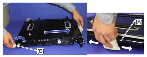
Put "Lubricant Powder" (B132 9700) on the surface of the image transfer belt [A], while you turn the drive gear [B] at a constant speed, as shown. (The straight arrow in the picture shows belt movement direction.) Lubricant powder prevents the image transfer cleaning blade from turning up.
