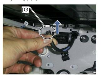
11. Keep the opening [G] of the toner supply tube up, and then clip the opening of the toner supply.
