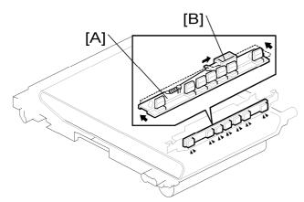
There are seven ID sensors. Three of them are for the line position adjustment. Four of them are for process control. The ID sensor shutter [A] covers the sensors when the machine is idle.
