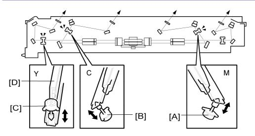
The WTL positioning motors for magenta [A], cyan [B], and yellow [C] adjust the angle of the WTL [D] respectively, based on the WTL position for black. This mechanism corrects main scan skew.
