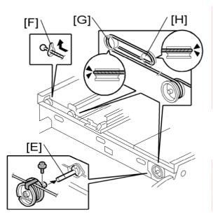
4. Install the drive pulley on the shaft [E].
