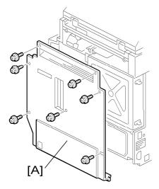
1. Remove the rear cover [A] of the machine ( $\Im x$  7).
