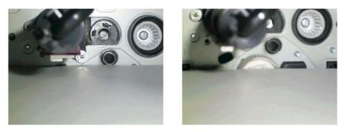
Make sure that a sheet of paper is attached to the frame of the rear side and covers the four gears. The picture on the left shows a sheet of paper that is correctly set, but the picture on the right shows a sheet of paper that is not correctly set. This sheet of paper prevents toner and screws from falling into the laser optics housing unit through cutouts.
