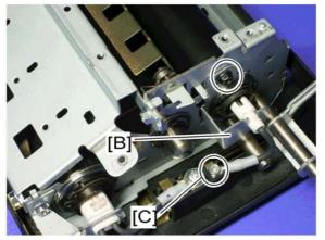
4. Pressure roller fusing lamp front stay [B] ( X 1) and screw [C] for the pressure roller lamp terminal
