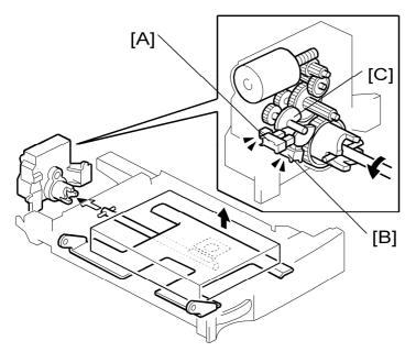
Two paper height sensors [A] [B] and actuator [C] are built into the paper tray lift motor. The paper height sensors, detect the amount of paper in the tray.
