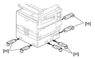
8. Attach the two caster stands [H] to the front, right, and rear sides of the machine.
