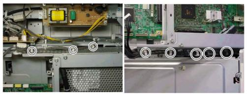
Release all the clamps on the top and bottom of the controller box (top: A 3, bottom: A 5).
