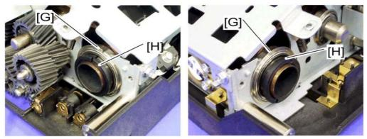
9. Remove the rear and front heating roller bearings [G] and insulating bushings [H].
