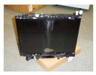
11. Put the front side of the image transfer belt unit on a corner of the table or a box as shown.
