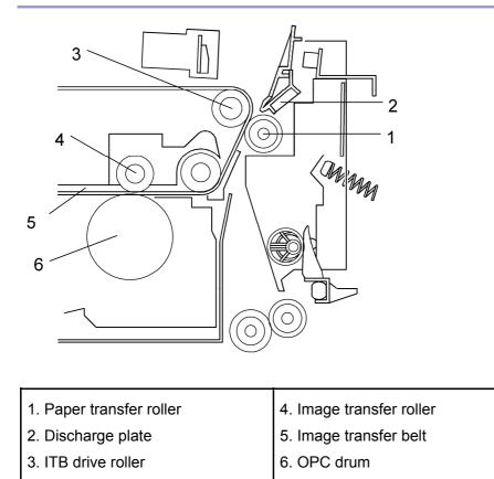
The paper transfer unit consists of the paper transfer roller and discharge plate. This unit completes the toner transfer to the paper.
