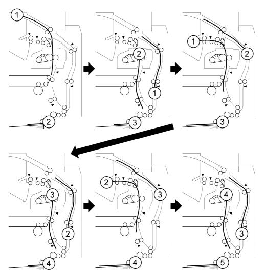
There are two sheets of paper in the paper feed path at the same time. The interleave method is used. For sheets longer than 400 mm, there is no interleaving.
