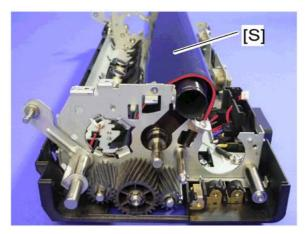
18. Fusing belt [S] with rollers (bearing x 4, insulating bushing x 2)
