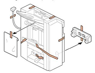
1. Unpack the finisher and remove all tapes and packing materials from the finisher.
