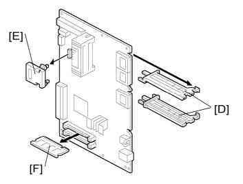
4. Interface rails [D], NV-RAM [E] and RAM-DIMM(s) [F]
