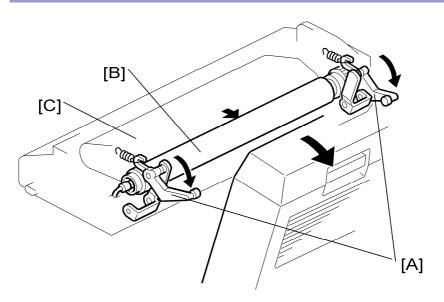
The pressure levers [A] put the proper pressure to the nip between the pressure roller [B] and fusing belt [C]. When releasing these levers, the pressure roller moves away from the fusing belt. If a paper jam occurs in the fusing unit, releasing these levers make jammed paper easily removed.
