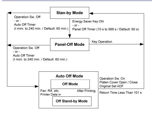
When the machine is not being used, the energy saver function reduces power consumption by decreasing the fusing temperature.
