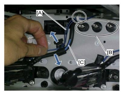
5. Release the harness [A] from the clamp (🛱 x 1 for YCM, 🛱 x 3 for K) and hook, and then disconnect the harness.
