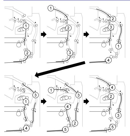
There are three sheets of paper in the paper feed path at the same time. The interleave method is used.
