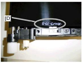
This belt must be installed the correct way around. When you reinstall the image transfer belt unit, install it with the painted number [D] on the belt at the rear side of the unit.
