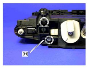
10. Remove the two screws and then front hold bracket [H] (as seen from the front).
