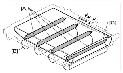
Each image transfer roller [A] applies current to the image transfer belt to attract the toner from each drum [B]. The high voltage supply board supplies current to the image transfer rollers and grounds the belt at roller [C].
