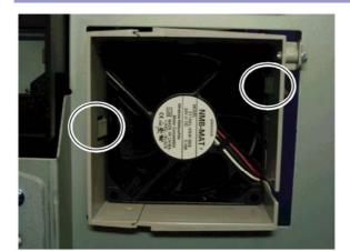
Make sure that the drive unit fan is installed with its decal facing to the right side.
