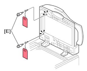
7. Remove two screws [E] from the bottom of the ARDF.
