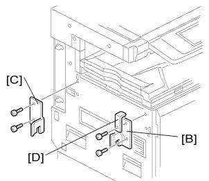
Install the front joint bracket [B], holder bracket [C] ( x 2 - M4 x 14), and rear joint bracket [D] ( x 2 - M4 x 14).
