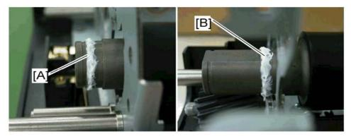
Apply "Barrierta S552R" to the front edge [A] and rear edge [B] of the pressure roller as shown above.
