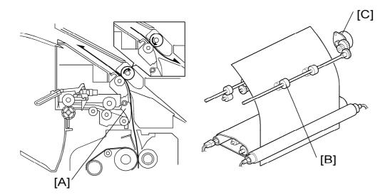
When paper is fed to the inverter tray, the junction gate [A] closes the paper path to the standard tray. And then, the inverter roller [B] feeds paper to the inverter tray. This roller is driven by the duplex inverter motor [C].
