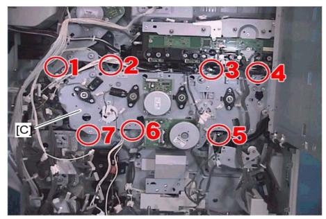
19. Gear unit [C] ( X 7, timing belt x 1)
