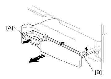
The lock at the front prevents the tray from coming out of the machine during transporting or shipping. When you pull the handle [A], the lock lever [B] is lowered. As a result, you can pull out the tray.
