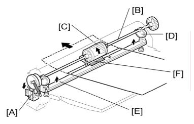
When the paper set sensor detects paper and the machine gets a by-pass printing job, the by-pass solenoid [A] unlocks the feed shaft stopper at the front end of the by-pass feed shaft [B].
