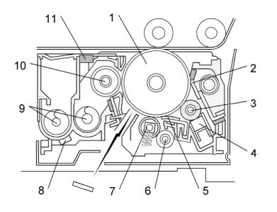
This machine has four tandem PCUs. Therefore, four color developments are possible during one paper path. This improves the productivity of outputs in color printing mode. Each PCU contains identical components (drum unit, development unit and so on), but the PCUs are not interchangeable.
