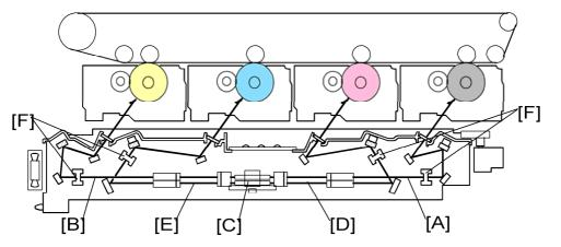
The laser beams for black [A] and yellow [B] are directed to the upper part of the polygon mirror [C]. Laser beams for magenta [E] and black [D] are directed to the lower part of the polygon mirror. The LD mirrors (see the previous page) deflect the laser beams for magenta and black towards the lower polygon mirror.
