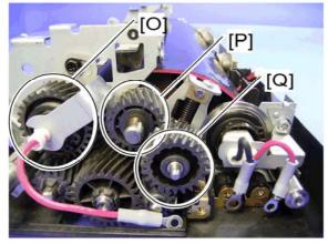
16. Remove the pressure roller gear [O] (C x 1), one-way clutch gear [P] (C x 1) and idle gear [Q].
