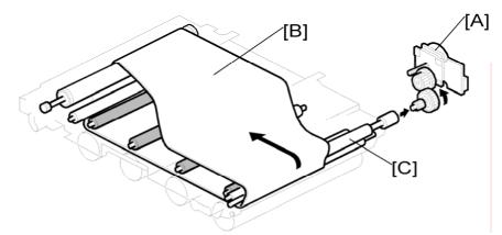
The ITB drive motor [A] drives the image transfer belt [B] and the cleaning unit via gears and the ITB drive roller [C]. The speed of ITB drive depends on the process line speed (see 'Laser Exposure – Optical Path').
