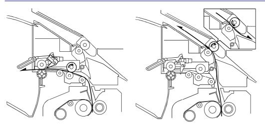
This machine uses the above switch back system for duplex printing. The drawing above right shows the paper feed for duplex printing.
