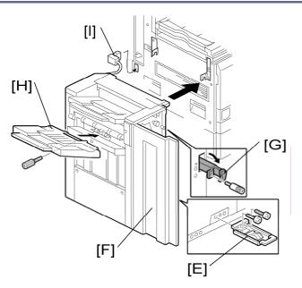
3. Install the grounding plate [E] on the finisher ( x 2 - M3 x 8).
