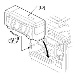
4. Install the 500-sheet finisher [D] on the machine ( $\square x$  1).
