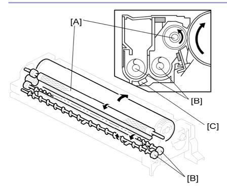
This machine uses a dual-component development system and has four development units (which are included in the drum units), one for each color. Each contains 225 g of developer when it is new. The developer in each unit is supplied to the development roller [A] by the two mixing augers [B] and attracted onto the surface of its roller.
