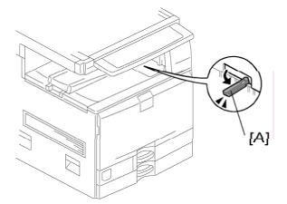
2. Pull out the feeler [A] for the output tray full detection mechanism.
