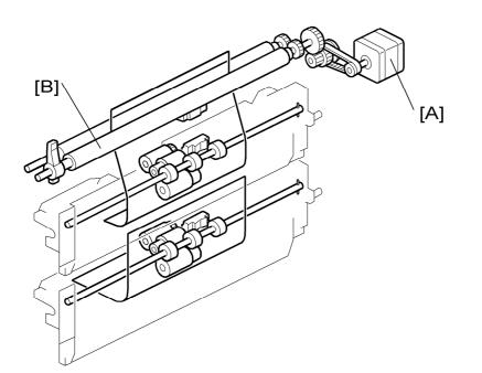
The registration motor [A] drives the registration roller [B] with a complex train of gears. The machine makes a paper buckle at the registration roller to correct paper skew. You can adjust the paper buckle with SP1-003.
