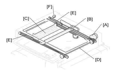
The scanner motor [A] drives the 1st scanner [B] and the 2nd scanner [C] through the scanner drive pulley, scanner drive shaft [D], and two scanner wires [E].
