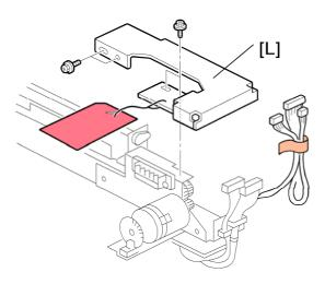
11. Remove the bracket [L] from the punch unit ( $\mathscr{F} \times 1$ ).
