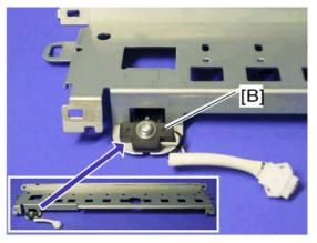
4. Heating roller thermistor [B] ( x 1)
