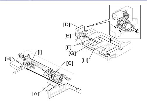
When the tray is installed in the machine, the tray bar [A] pushes the lever [B], and this lever pushes down the pick-up roller [C] onto the paper.
