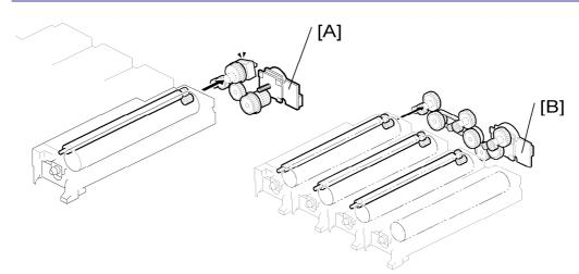
The drum/development drive motor-K [A] drives the development roller for black through gears and a clutch. The gear trains are shown in the diagram.
