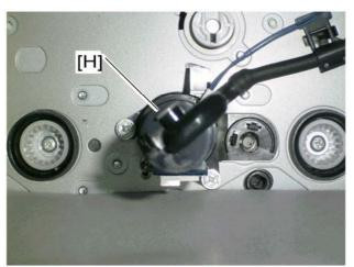
8. Insert the toner pump unit [H] into the rear frame of the machine ( $\mathscr{F} \times 2$ ).
