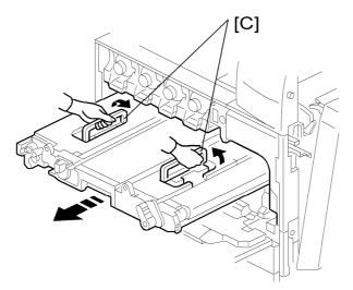
6. Grasp the handles [C], and then pull out the image transfer belt unit fully.
