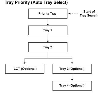
The "Tray Priority" setting determines the start of the tray search when the user selects "Auto Tray Select" with the driver. The machine searches paper trays for the specified paper size and type.
