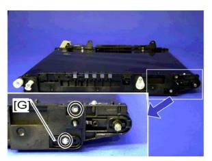
9. Remove the two screws and then rear hold bracket [G] (as seen from the rear).
