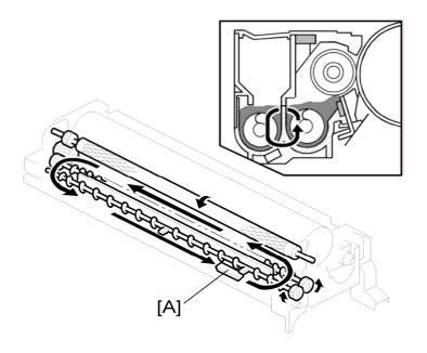
The TD sensor [A] in the development unit has an ID chip that contains the new unit detection flag. The machine detects that a PCU is new if the flag in the ID chip is activated. The machine automatically does the following adjustments when detecting the new unit detection flag.
