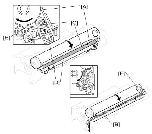
The cleaning blade [A] scrapes off the used toner that stays on the drum. The toner collection auger [B] transports the used toner towards the toner collection duct. Then it goes to the toner collection duct. The brush roller [C] put lubricant on the drum to make toner removal easy the next time the drum rotates past the cleaning blade.
