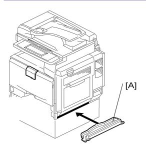
When the copier is installed on the floor without the optional paper tray unit or a table, the cover [A] must be attached to the copier.
