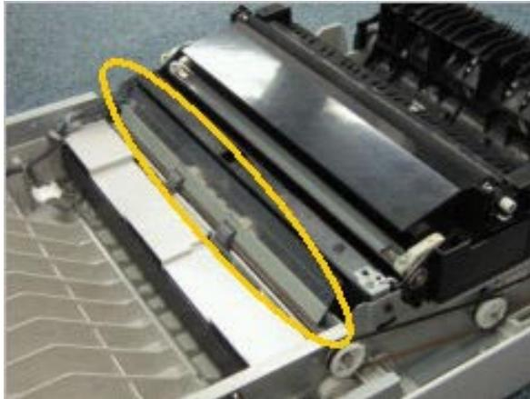
1. Remove the duplex unit (see Service Manual, Replacement & Adjustment).
