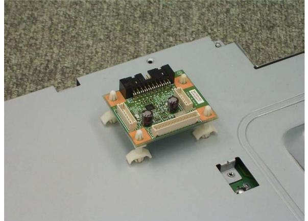
7. Connect one end of the harness to **CN3** on the **key counter I/F board**, and the other end to **CN252** on the **IOB board**.
