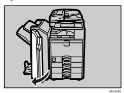
**2** Pull out the punch waste box carefully, and then remove punch waste.
