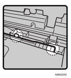
To detach the cleaning brush, release the catch at the center of the cleaning brush, hold the catch to prevent it re-engaging, and then raise the cleaning brush grip.
