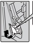
1.Open the front cover of the finisher, and then pull out the staple unit.
