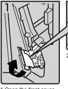
1. Open the front cover of the finisher, and then pull out staple unit.
