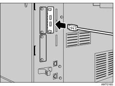
Secure the USB cable using the hook.
