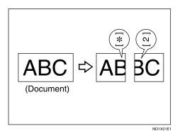
For example, this function splits the document if the document length is 20 mm (0.79") or longer than the paper used. The document is reduced if it is less than 20 mm (0.79"). When a document is split, an asterisk ( $\frac{\textbf{X}}{\textbf{X}}$ ) is inserted at the split position and about 10 mm (0.39") of the split area is duplicated on the top of the second sheet.
