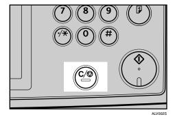
Pressing the [Clear/Stop] key deletes by single digits the fax number or IP-Fax address. The Internet Fax address can be entirely deleted at once by pressing the [Clear/Stop] key.
