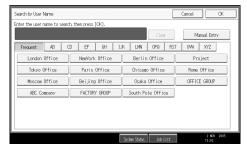
To search by directly entering a user name, press [Manual Entry], and then enter the user name. Partial matching is used when searching for a user name.
