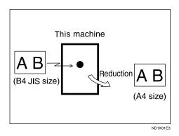
If you turn this function on, the machine reduces the width and length of the received image so that it will fit on one page. If  $A4\Box$  paper is loaded and a document of B4 JIS $\Box$  size is received, the machine will reduce the document to a single  $A4\Box$  sheet.
