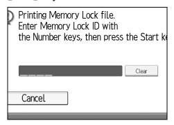
If the Memory Lock ID does not match, the "Specified code does not correspond to programmed Memory Lock ID." message appears. Press **[Exit]** and retry after checking the Memory Lock ID.
