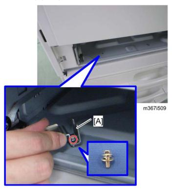
10. Attach a screw (spring washer screw), using a securing bracket [A] to tighten the screw.
