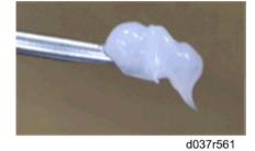
7. Apply a small amount of "Silicone Grease G501" to the gear of the motor as shown above.
