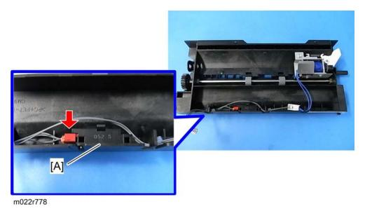
2. Fusing exit sensor [A] ( $^{\square}$  x 1, hook x 1)
