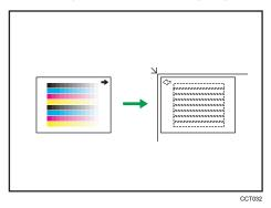
Make sure to set the test pattern on the exposure glass, and then two or three white sheets, same size
