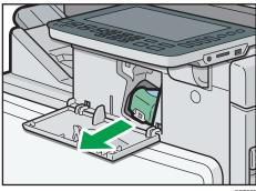
4. Open the face plate of the cartridge, and then remove any jammed staples.
