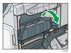
4. Remove the misfed paper, and then return the cover C to its original position.
