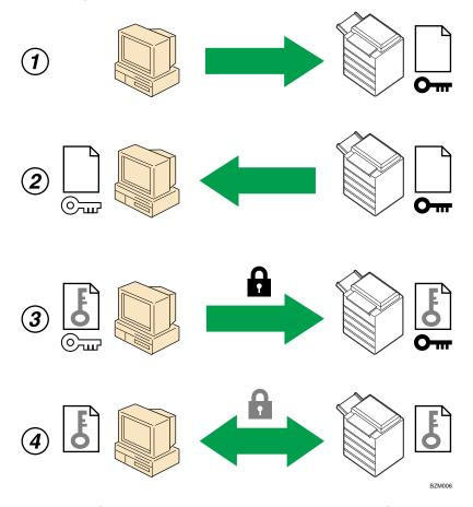
1. To access the machine from a user's computer, request the SSL device certificate and public key.
