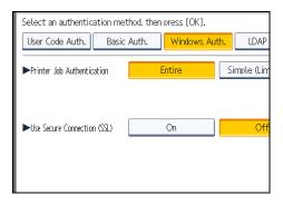
If you are not using secure sockets layer (SSL) for authentication, press [Off].
