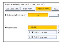
To enable Kerberos authentication, a realm must be registered beforehand. The realm name must be registered in capital letters. For details about registering a realm, see "Programming the Realm", Network and System Settings Reference.
