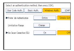
If you are not using secure sockets layer (SSL) for authentication, press [Off].
