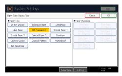
Press [Do not Display] on the [Paper Type] area, and then press [Thick Paper 1], [Thick Paper 2], [Thick Paper 3], [Thick Paper 4], or [Thin Paper] on the [Paper Thickness] area when loading thick paper or thin paper.
