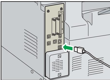
**2. Connect the other end of the USB interface cable to a card authentication device or media slot.**
