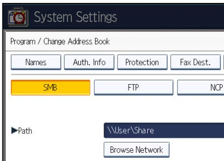
If the network does not allow automatic obtaining of IP addresses, include the destination computer's IP address in the path. For example: if the IP address of the destination computer is "192.168.0.191", and the folder name is "Share", the path will be "\\192.168.0.191\Share".
