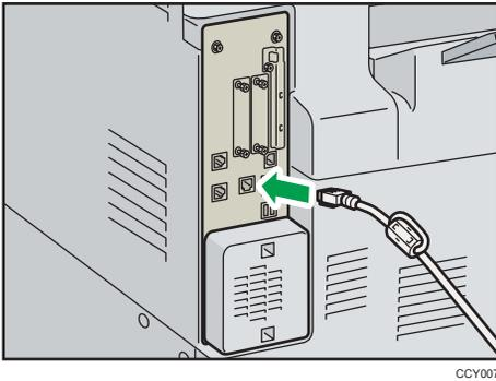
4. Connect the other end of the Ethernet interface cable to a network connection device such as a hub.
