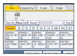
Press the transmission type tab to switch the transmission type between fax/IP-Fax, Internet Fax, email, and folder.
