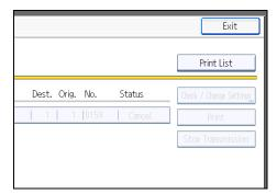
After pressing [Check / Stop Transmission File] under [Change TX / Info] in step 1, press [Exit] twice. The standby display appears.
