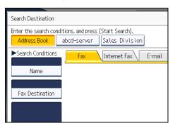
3. Press the transmission type tab to switch the transmission type to fax/IP-Fax, Internet Fax, e-mail, or folder.
