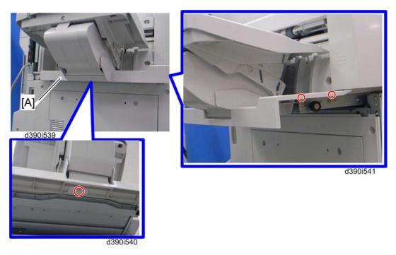
4. Remove the output tray lower cover [A]; this cover is for the internal finisher without the punch unit ( $\mathscr{F} \times 3$ ).
