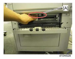
4. Press the surface of the vertical transport roller [A] for the tray 2 gently with a small piece of paper, as shown above.
