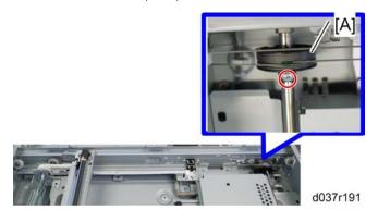
10. Rear scanner drive pulley [A] (  $\mathcal{F}$  x 1)
