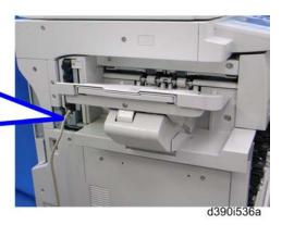
3. Attach the bracket [A] (  $\mathscr{F}$  x 2); this bracket is for the internal finisher when used with the punch unit.
