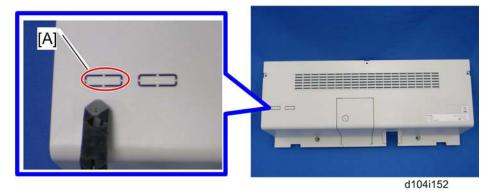
4. Remove the cutout [A] in the rear lower cover with nippers.
