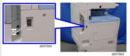
[2] Finisher: Rating voltage output connector for accessory Max. DC24V
