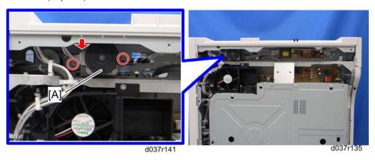
2. Scanner motor assembly [A] ( Fx 2, spring x 1, 🖾 x 1, timing belt x 1)
