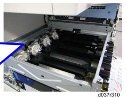
4. Take aside the ITB contact motor unit [A] (  $\mathcal{F}$  x 2)
