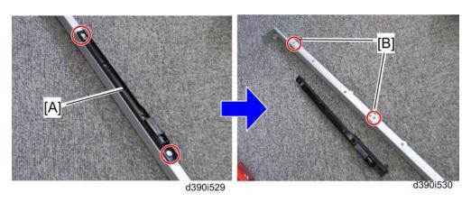
4. Remove the stopper [A] from the guide rail, and then attach with the screw holes [B] (these screw holes must be used when the internal finisher is installed with the punch unit).
