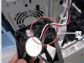
Make sure that harnesses are correctly set [A] along the guide on the fan frame without slack [B]. Otherwise, the some of the wires could be pinched and damaged or cut between the fan frame and the frame of the main machine. SC533 can be issued if the harnesses are broken.
