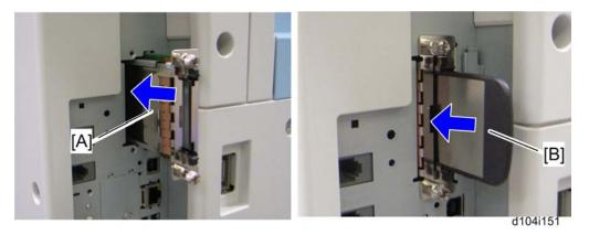
2. Install the Bluetooth board [A] (Knob-screw x 2) into the slot.
