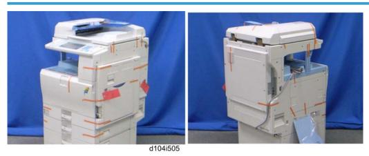
1. Remove all the tapes and retainers on the machine.
