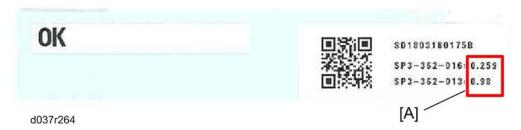
3. Input all correction coefficients [A] for the ID sensor with the SP modes referring to the barcode sheet provided with the new ID sensor unit/board.
