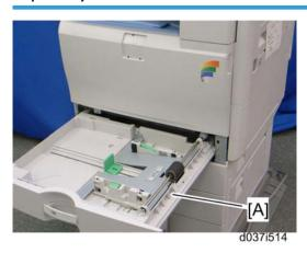
1. Pull each paper tray [A] out. Then adjust the side guides and end guide to match the paper size.
