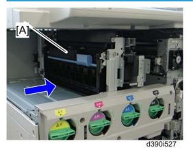
1. Install the punch and inverter unit [A] in the mainframe.
