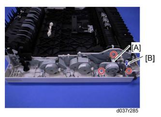
3. By-pass motor with the bracket [A] ( 🗗 x 3, 😂 x 2, 🚅 x 1)
