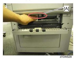
7. Press the surface of the vertical transport roller [A] for the tray 2 gently with a small piece of paper, as shown above.
