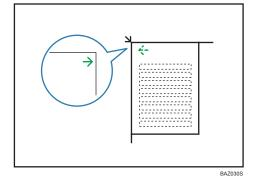
• Make sure to set the test pattern on the exposure glass, and then two or three white sheets, same size as the test pattern, above the test pattern.
