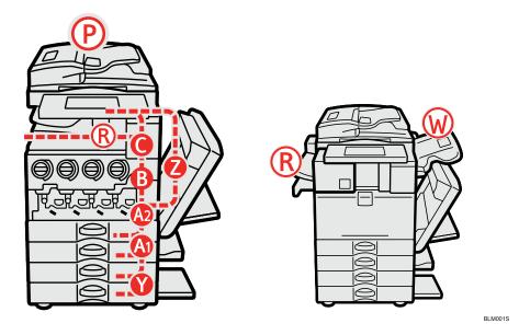
1. Press the key of the section from where you want to remove the jammed paper.
