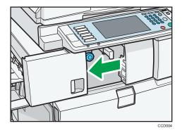
3. Pull out the punch waste box carefully, and then remove punch waste.
