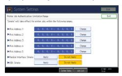
You can specify the IPv4 address range to which this setting is applied, and whether or not to apply the setting to the parallel and USB interfaces.
