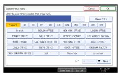
To search by directly entering a user name, press [Manual Entry], and then enter the user name. Forward matching is used when searching for a user name.
