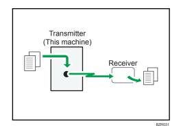
Normally the machine is in the Memory Transmission mode. To switch the mode to Immediate Transmission, press [Immed. TX].
