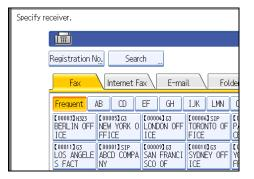
Press the transmission type tab to switch the destination between fax number, Internet Fax destination, e-mail address, and folder destination.
