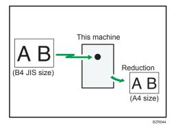
If A4 paper but not B4 paper is loaded and a B4<sup>D</sup> document is received, the machine automatically reduces the document size so that it can be printed onto a single A4 sheet.
