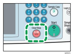
The machine stops scanning.
