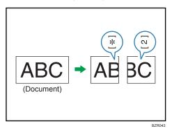
For example, this function splits the document if the document length is 20 mm (0.79 inch) or longer than the paper used. The document is reduced if it is less than 20 mm (0.79 inch). When a document is split, an
