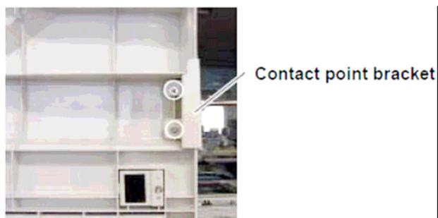
6. Attach the rise handle bracket to the upper right edge on the inside face of the ADF cover (binding screw x 2).
