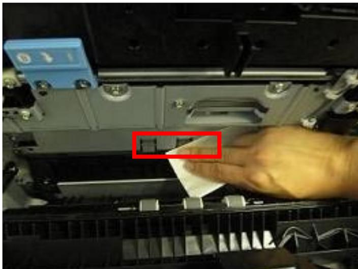
5. If Jam 17 still occurs, turn the paper feed motor using **SP5-804-009** (Output check: Paper Feed M2: CW:190mm/s).
