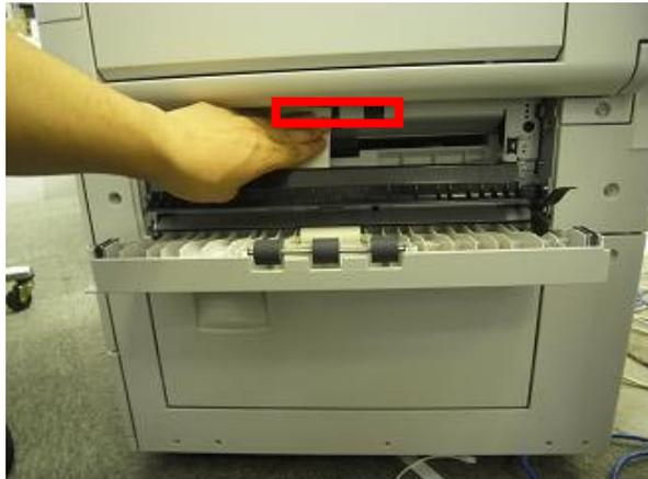
5. If Jam 11 still occurs, replace the brackets for the vertical transport covers (Front: P/N D0392943, Rear: P/N D0392944).
